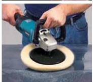
Start with the Super Cut Wool Pad. (Spur wool pad before starting to condition and remove loose yarns or dry polish). Apply Liquid Ice Extra-Cut to the work area and spread with the pad before starting the machine. Buff using medium pressure at 1000 –1200 rpm. Remove all sand scratches before moving to pad #2.
