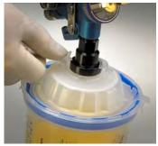
"Snap" the adapter locks over the adapter base to secure the lid to the gun adapter.
