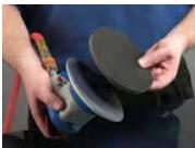
Apply the thin interface pad to the back-up pad.
