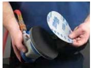
Apply a P1500 grit disc to the thin interface pad.
