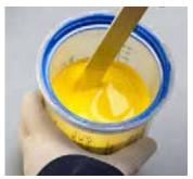
Mix paint by stirring (if not using a shaker) and clean liner flange/ring area of any paint before attaching to lid.
