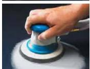
Start the D/A after it is in contact with the surface. Use light pressure. Work in small sections with a slow, steady movement. Sand in an up and down motion then traverse using a side to side motion.
