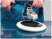
On dark finishes the White Finishing Foam Pad is recommended to remove the finest polish swirl marks and produce a high gloss finish. Buff at 1500 rpm.
