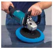
Use the Blue Cutting Foam Pad and follow the same procedure, except turn the buffer rpm up to 1500. Remove all polish swirl marks before moving to pad #3.
